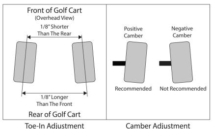
2. Adjust the toe by loosening both driver and passenger side jam nuts. Lengthen or shorten the tie rod by turning the rod adjustment. Shortening the tie rod increases the toe-in, lengthening decreases it.
