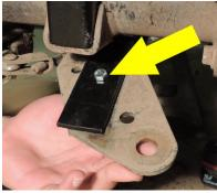
Fasten the centering plate assembly to the rear axle, riser block, leaf spring and new shock mounting bracket using (2) <u>7/16-14 x</u> <u>7.25" Hex Head Bolts</u>, (4) <u>7/16 Flat Washers</u> and (2) <u>7/16-14 Nylock Nuts</u>. Hand tighten.
