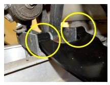
Reinstall the (3) tie rod ends onto the spindles using the original hardware. If the safety pin hole is not entirely visible through the castle nut's gaps, keep tightening.
