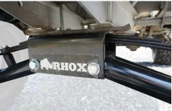
Using (4) <u>10mm x 50 Serrated</u> <u>Flange Head Bolts</u>, (4) <u>10mm Flat</u> <u>Washers</u> and (4) <u>10mm Nylock</u> <u>Nuts</u>, bolt the new BMF front suspension to the chassis where the original suspension was removed.
