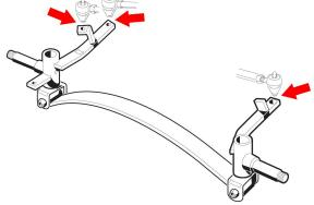
12. Disconnect the bottom of the shocks from the A-Arms. Discard hardware. Push the shock up and out of the way.
