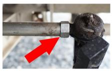
3. Adjust the camber by changing the position of the camber adjustment bolts on the upper A-Arms.
