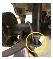
2. With the axle supported by the jack, remove the (2) nuts holding the driver's side U-bolt around the rear axle, leaf spring and shock mounting plate. Remove and discard hardware.
