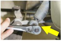
13. Disconnect the lower portion of the A-Arms from the spindles and discard hardware. Disconnect the upper portion f the A-Arms from the frame. Discard the A-Arms but retain the hardware and the A-plate straps (blue).
