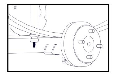
NOTE: The axle alignment bolt in the leaf spring is not centered and should be offset further to the rear of the vehicle. If installed backwards the rear axle will push too far forward and cause tires to rub against tire well.
