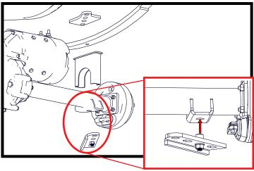
NOTE: The 16-051 lift kit only uses the short blocks which have no angle.
