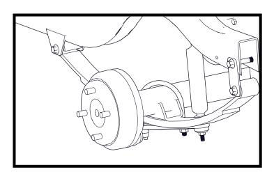
**NOTE:** Failure to support rear axle with floor jack could potentially damage rear end.
