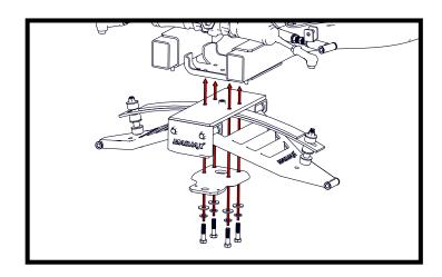
NOTE: DO NOT adjust the bushing assemblies at the end of the leaf springs. These bolts are preset to the proper tightness. It will not appear tight until the weight of the vehicle is on the suspension.
