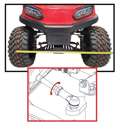
Drive vehicle a short distance to allow new components to settle and then re-check camber and toe measurements again. If needed, adjust accordingly by adjusting camber first before toe, using steps above. Retighten all hardware.
