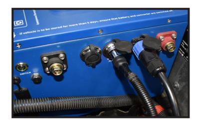
Plug the Low Battery Buzzer harness into the outlet labeled "BUZZER GAUGE" on the battery case.
