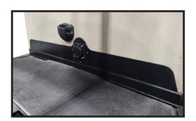
Plug the lithium charge port into the corresponding plug from the on board charger.
