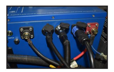
Coil any excess harness or cable together and secure with a zip tie inside the battery tray.
