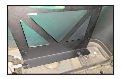
Install two (2) threaded clips to the base of the mounting tray. The threaded portion of the clips will be on the top.
