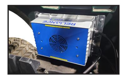
Plug the charge port cord into the appropriate plug coming from the onboard charger.
