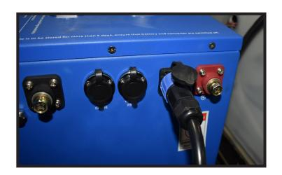
Plug the dash harness into the outlet labeled "KEY/ CAN" on the battery case.
