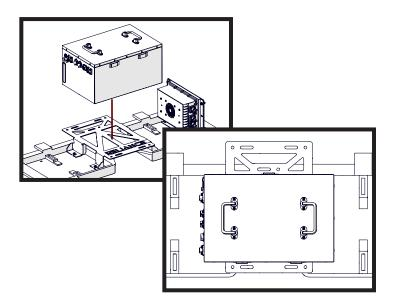
Install a J-hook into the base bracket as shown. Be sure that the J-hook mounting hole is below the corresponding retaining bracket on the battery case.
