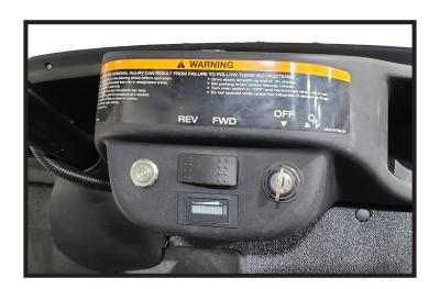
Plug the dash harness into the back of the power buton.
