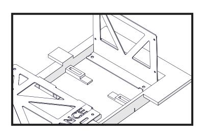
Install two (2) threaded clips to the base of the mounting tray. The threaded portion of the clips will be on the top.
